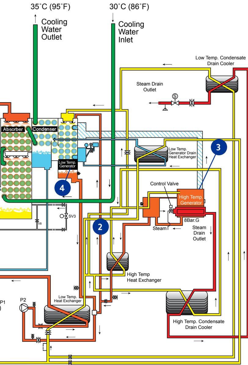
**2. Parallel flow cycle** divides the solution flow between the low-temperature and high-temperature generators into two parallel, balanced paths. The result is safer and more efficient operation at a much lower pressure than conventional series-flow designs.
